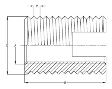
Female thread A = M27 Length B = 30 Male thread E = 34.0 Min hole depth blind hole = 36
